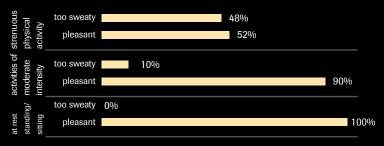
**TEMPERATURE** inside the test boots (outdoors, at different activity levels):
